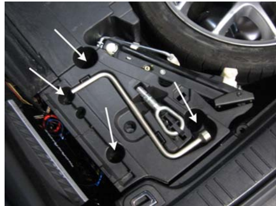
Remove the four 10mm nuts and lift the panel upward.
